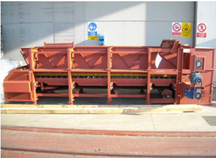
CNG Box Rubber Feeder
