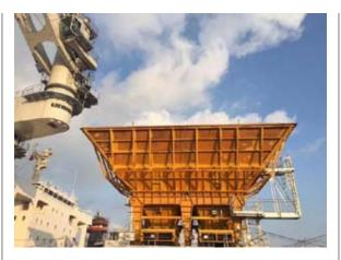
The TV transfers the coal from the OGVs into barges, which then transport the coal to the port for discharge.
