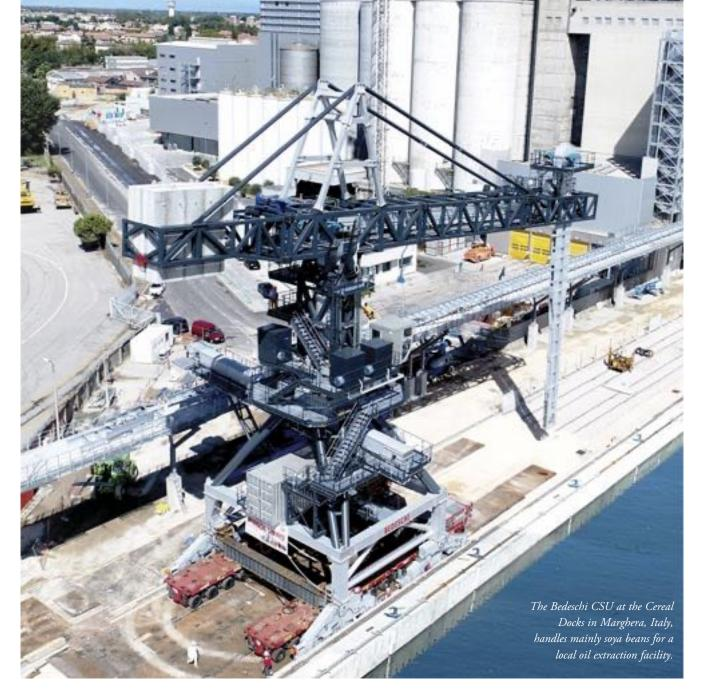
bases its unloading system on the proven chain elevator technology, which grants lower power consumption, gentle handling of the material, and simple and inexpensive maintenance.
