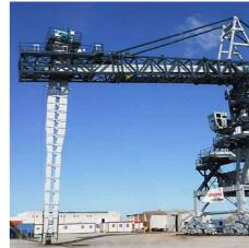
Ship loader - Ship unloader Travelling, tower, luffing and slewing SHL - Any type of material from coal to grain - Continuous ship unloader Environmental friendly solutions
