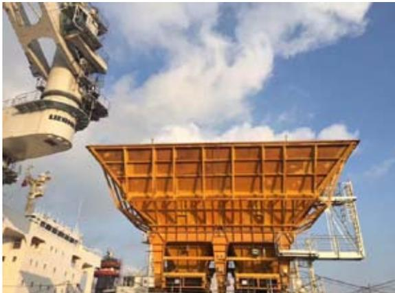
The TV transfers the coal from the OGVs into barges, which then transport the coal to the port for discharge.
