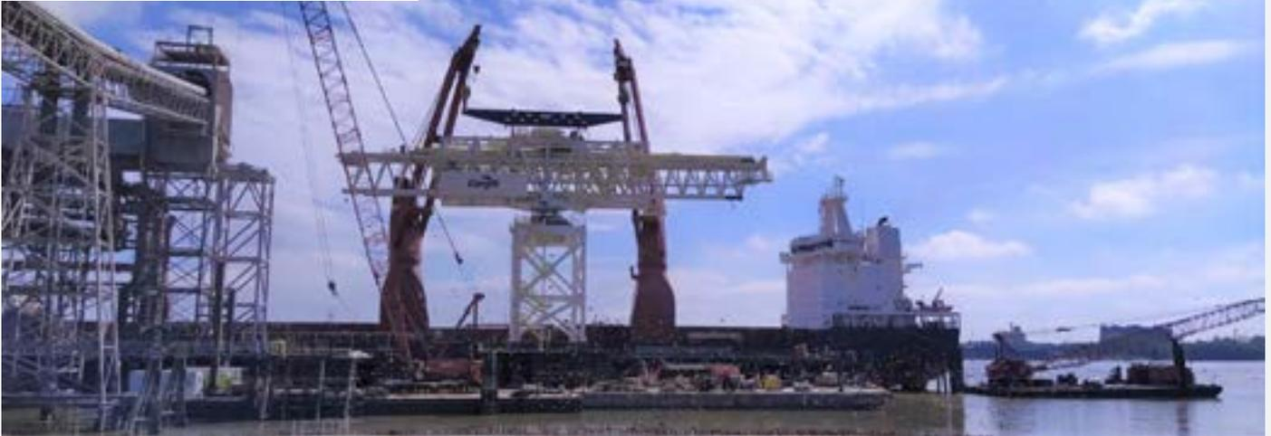
After a ship's hold is full, the loader moves on to the next operating zone, travelling at a rate of approximately 40m per minute.
